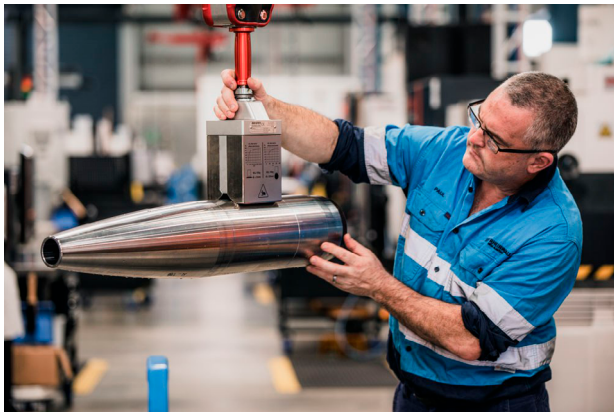
Figure 5: A 155-mm projectile on NIOA's Maryborough, Queensland, production line; NIOA is now producing munitions for the ADF and for export to Australia's partners overseas
