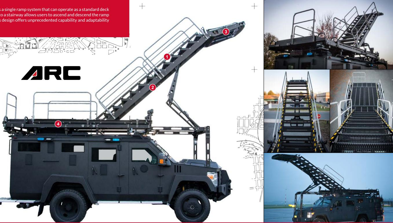
The RAID Elevated Tactics System is a complete package that includes a customized, heavy-duty jump out van with a Liberator, Side Assault System, and Side Deployment Rail. This versatile, multi-purpose tactical deployment and transport system supports teams of up to 10 people.
